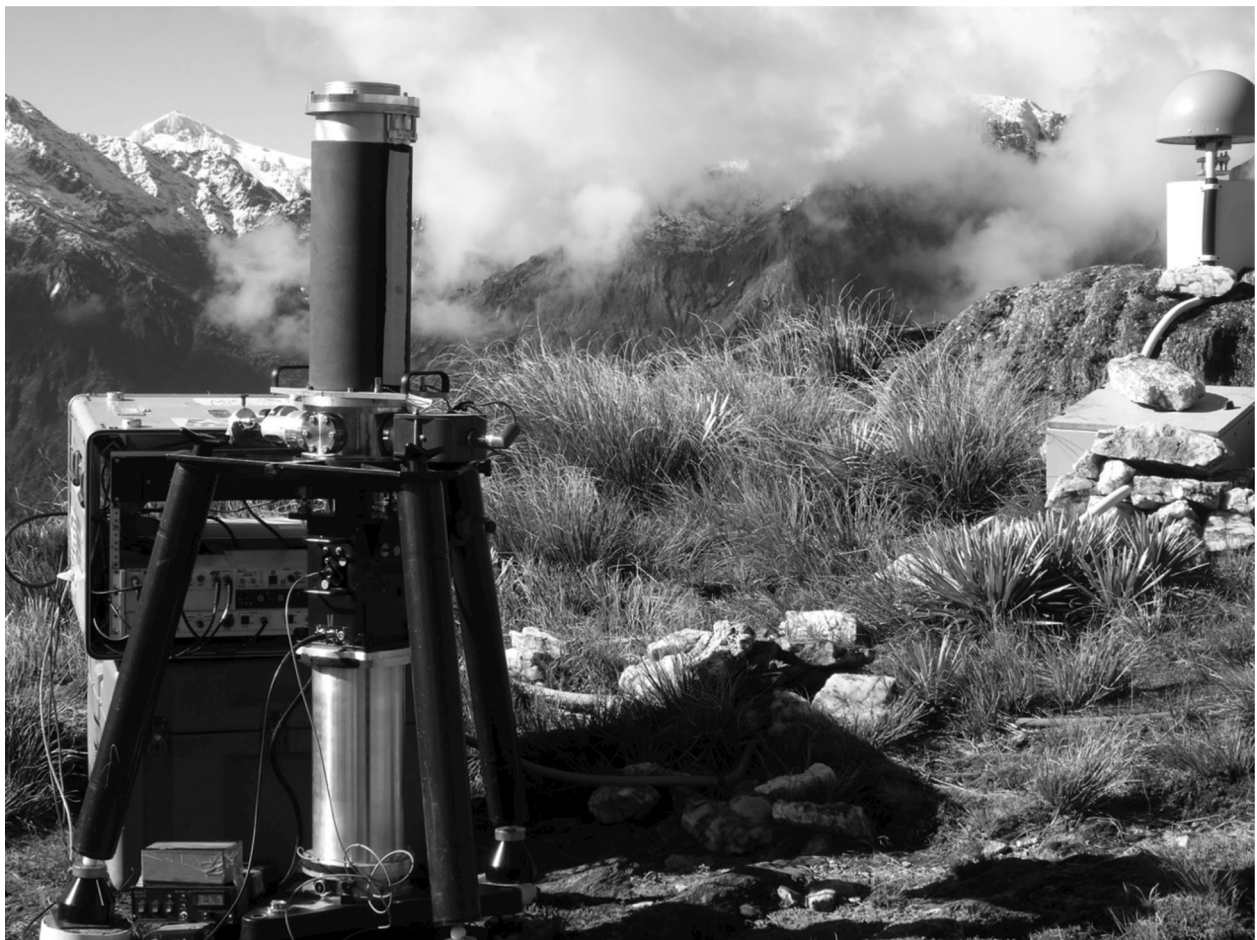
Figure 2. FG5 absolute gravimeter set up at Leo Creek prior to erecting the instrument tent. The higher cylinder is the evacuated dropping chamber, and the lower cylinder houses a spring-mounted inertial mass to isolate the instrument from microseisms. The electronic control module is housed in the large box behind the gravimeter. The dome and antenna mount of the Leo Creek GPS point is visible extreme right. Water level fluctuations in a small lake below and 100 m north of the point may be responsible for unmodelled gravity changes between 2000 and 2015.
